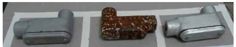
Before and after photographs. Above photo are new conduit bodies and below photo shows same conduit bodies after 42 days in salt fog
