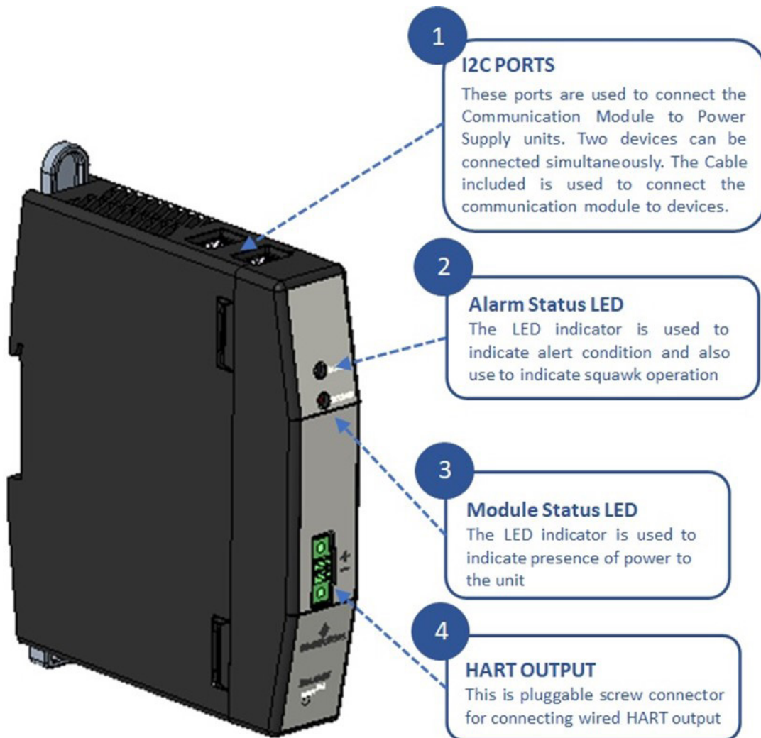
Figure 1.3: Parts of the HART Communication Module
