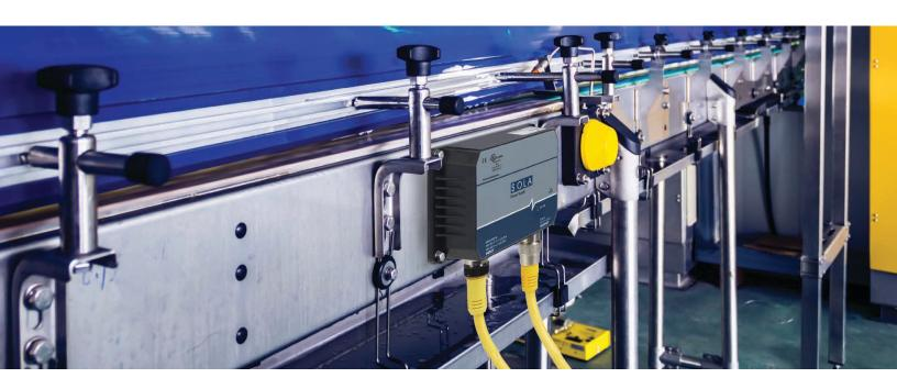
SolaHD IP67 SCP-X power supplies mount directly to your machine or production line, eliminating the complexity and cost of unnecessary enclosures and excess wiring.
