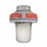
Class I, Division 1 explosion proof luminaires have engineered flamepaths that vent the pressure of an explosion and release cooled gases at temperatures that will not ignite the surrounding flammable atmospheres.
