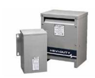
Transformers address variable speed motor drive applications to magnetically isolate the motor drive from the main plant power. Drive isolation and K-factor transformers can be used with DC drives or variable-frequency AC drive applications to change voltage, reduce drive-induced ground currents, and reduce common-mode noise.
